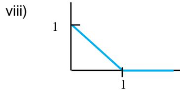
2. Referring to the Laplace transform table, find the transform  $\mathcal{L}\{f(t)\}$ . Show the modification details that you need to do before the transform can be done.
