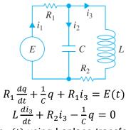
$L\frac{di_3}{dt} + R_2i_3 - \frac{1}{c}q = 0$  Find the charge on the capacitor q(t) using Laplace transform when L = 1H,  $R_1 = 1\Omega$ ,  $R_2 = 1\Omega$ , C = 1F,  $E(t) = \begin{cases} 0, & 0 < t < 1 \\ 50e^{-t}, & t \ge 1 \end{cases}$ ,  $i_3(0) = 0$ , q(0) = 0.
